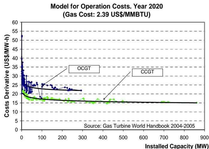
Figure 6: Short Term Marginal Cost (STMC) for Generators.
