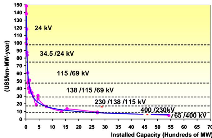
Figure 4: Annualized Long Term Marginal Cost per length unit (ALTMC) for Transmission Lines.
