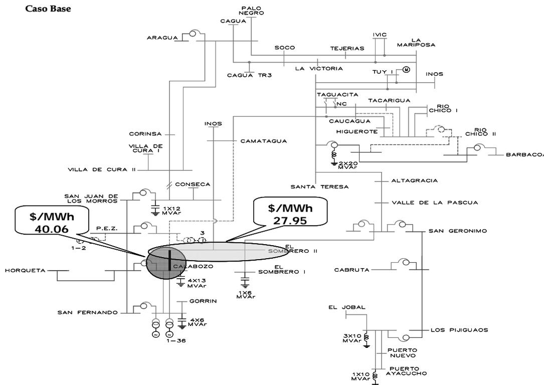
**Figure 8: Addition of a new link between El Sombrero II 115 kV and Calabozo 115 kV following the sensitivities to nodal Active Power Balance in the Venezuela Mid-eastern power system.**
