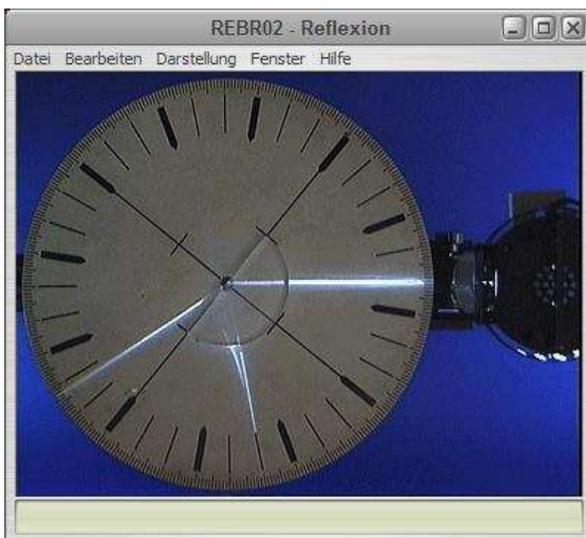
Figure 3. Screenshot of a remote experiment used during exam, showing critical angle phenomena.
