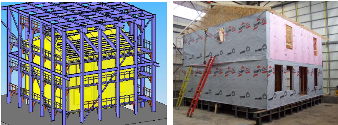
Figure 7: 3D CAD drawing of the two-storey test house with the reaction frame surrounding it (left) as well as a photograph of the house in December 2005 (right).
